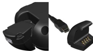
If placing to charging cradle, place first the bottom towards the charging pins in the cradle and the let the top of the unit lie down.
